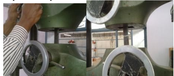
Fig.4. Specimen under tensile test
