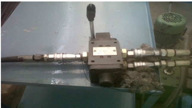
Figure 4.4: Hydraulic Lever o Maintain Pressure
