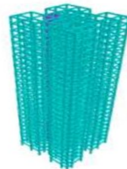
Fig 3.3: G+26 RCC Shear Wall Structure with different shear wall location
