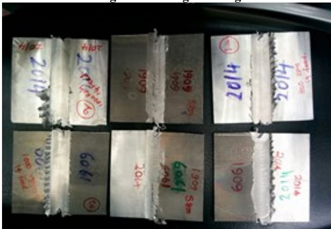
Fig.3.4: Welded Specimens at different speeds and feed rate
