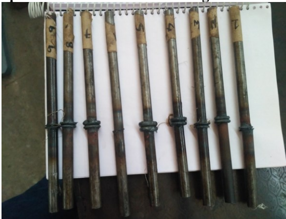
Figure 4.6 Specimens after friction Welding
