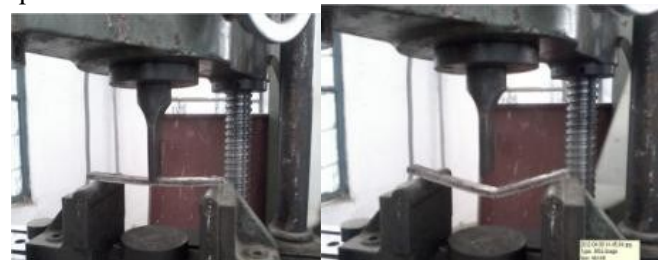
Fig.5. Specimen under the 3 point bending test
